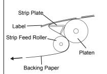
3. If the peel-off issue is performed under intense light, the strip sensor may not correctly detect the presence of a printed label on the strip shaft. In this case, reduce the intensity of the light or fit the Shade Plate to the Strip Block as shown in the figure.
